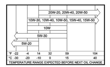
**NOTE:** The use of less than service class SH oil or extending the oil change intervals longer than recommended can result in engine damage.
