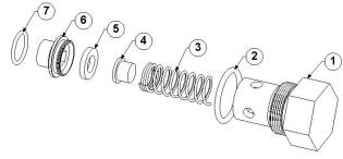
23-023 VLV, CHECK, CHECK VLV MANIFOLD
