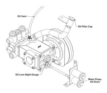
2. After the first **50 hours** of operation, change the crankcase oil with CAT Pump Crankcase Oil, (Part # 13-000). Change the crankcase oil every **500 hours** thereafter.
